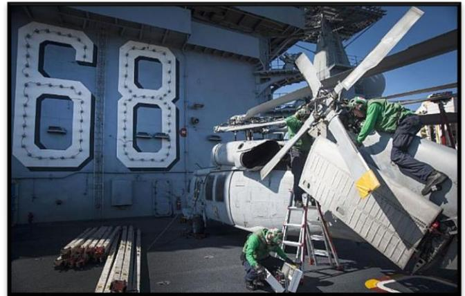
**Figure 8.** Sailors perform maintenance on the propeller of an MH-60S Sea Hawk helicopter assigned to the Eightballers of Helicopter Sea Combat Squadron (HSC) 8 on the flight deck of the aircraft carrier USS Nimitz (CVN 68)
