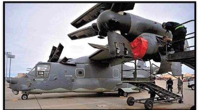
**Figure 6.** Airmen perform maintenance checks on a CV-22, tilt-rotor aircraft Osprey on the flight line at Cannon Air Force Base.
