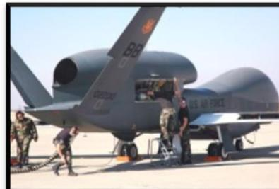
Figure 3. Avionics specialists with the 12th Aircraft Maintenance Unit prepare a Global Hawk for a runway taxi test at Beale Air Force Base, California.
