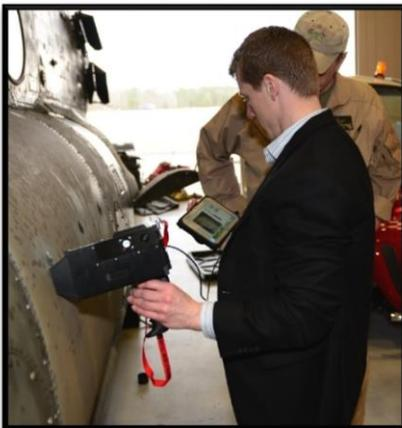
**Figure 4.** LPT-S2 system in use, with main instrument housing and tablet PC display shown.
